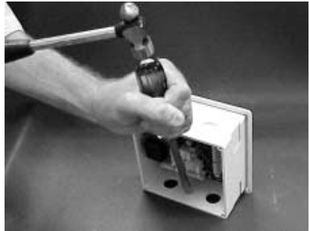
FIGURE 3-1. Removing the Knockouts
