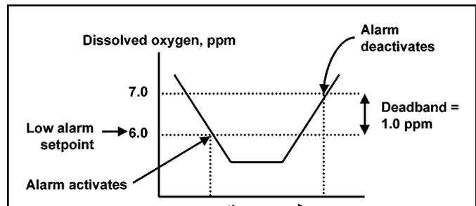
**FIGURE 5-3. Low Alarm Logic**
