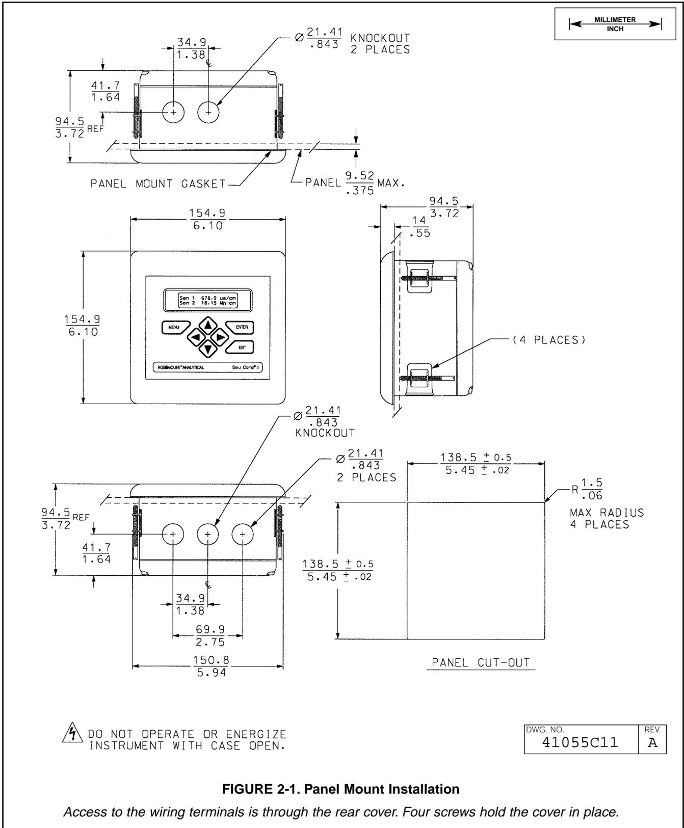
FIGURE 2-1. Panel Mount Installation
