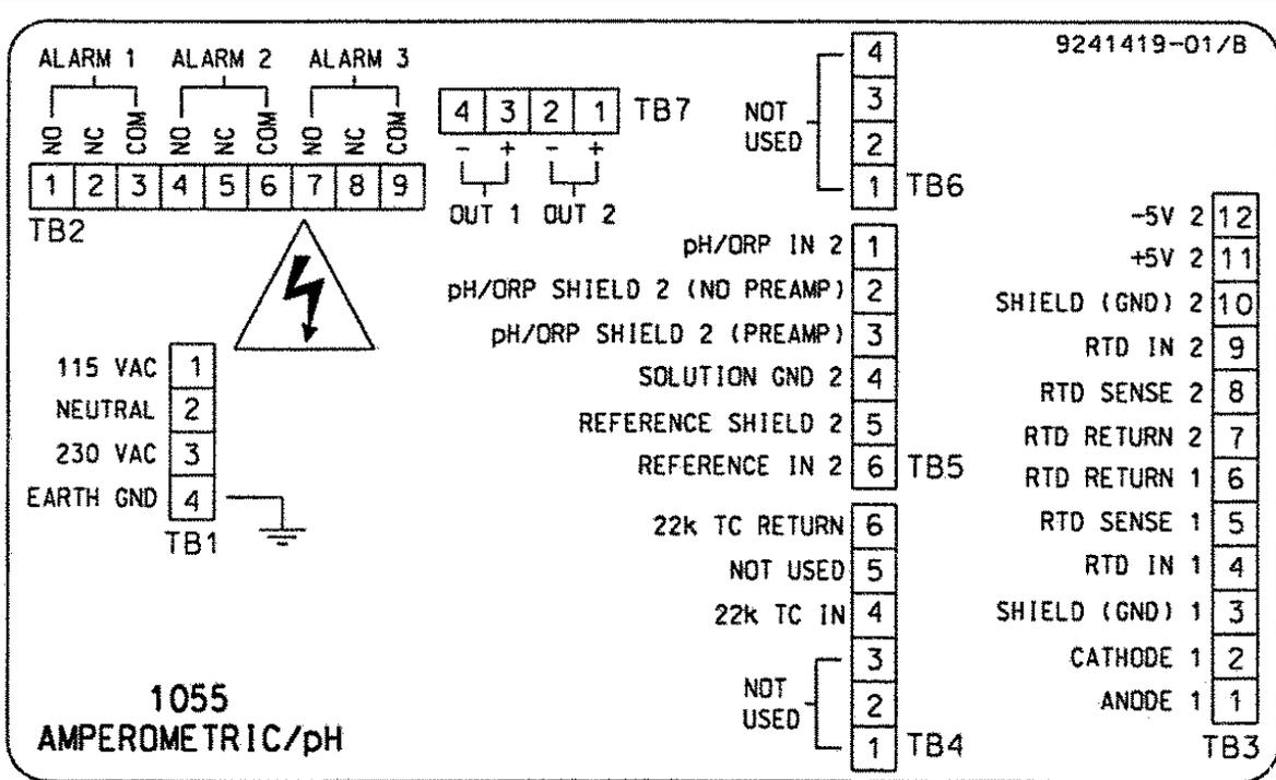
FIGURE 3-4. Wiring Connections for Model 30-B-PH/DO
