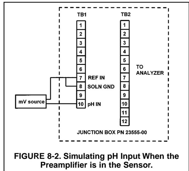
**FIGURE 8-2. Simulating pH Input When the Preamplifier is in the Sensor.**
