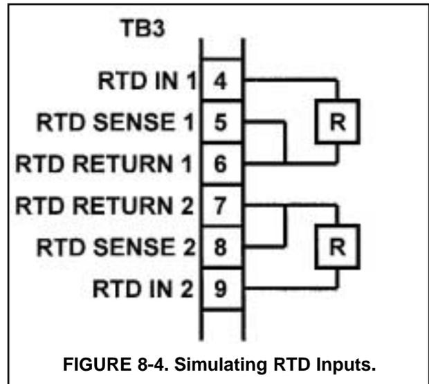
FIGURE 8-4. Simulating RTD Inputs.
