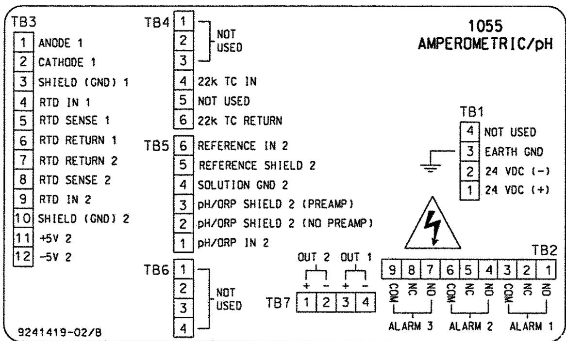
FIGURE 3-3. Wiring Connections
