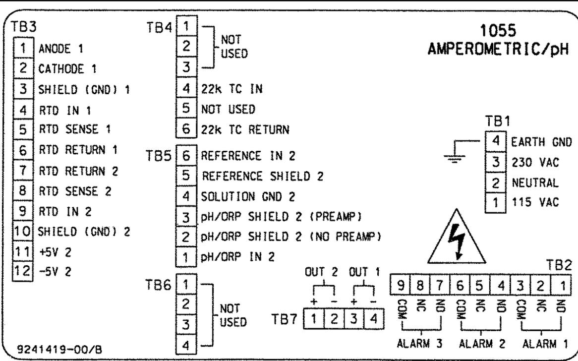
FIGURE 3-2. Wiring Connections for Model 30-A-PH/DO
